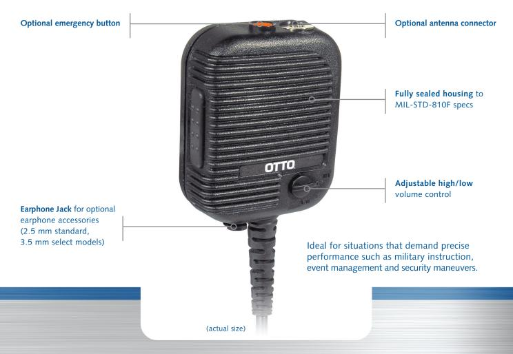
The **Evolution speaker microphone** is compatible with a variety of radio makes and models and has a tailored, environmental design that offers both mobility and stability during routine or vigorous conditions. The preferred remote speaker microphone for the public safety sector, it is also used by military forces, government security and military police who depend on ultimate clarity and calculated safety for training exercises, event coordination detail, and high security operations.
